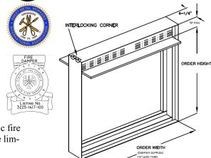
TOP BLADE RIVETED TO FRAME
